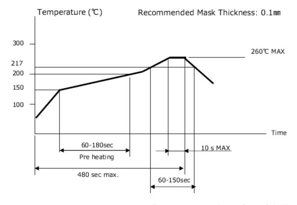
Temperature on the surface of PWB
